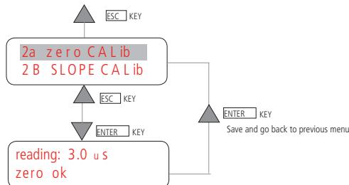
Select "2B SLOPE CALIB" for Slope calibration. Set buffer solution value (0 to 99.9  $\mu$ S).
