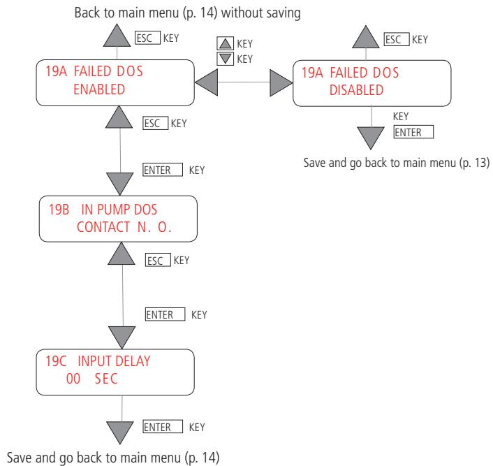
If a pump alarm occurs, if PUMP DOS. IN contact is enabled, instrument shows “SYSTEM WAITING - FAILED DOSAGE” and alarm output is active.
