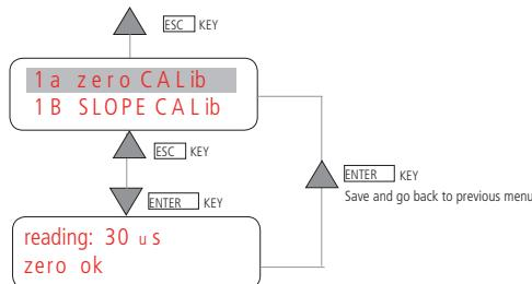
Select "1B SLOPE CALIB" for Slope calibration. Set buffer solution value (0 to 999  $\mu$ S).
