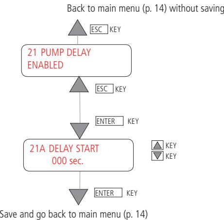
If a delay is set, after electrovalve start the instrument shows:
